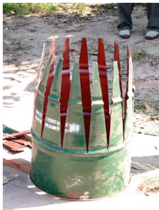
Funnel-shaped fuel silo from a 200-litre oil barrel
