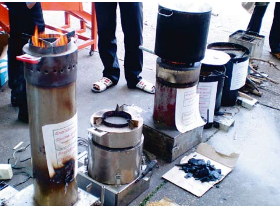
“High-end” versions of the rocket stove – cooking using rice husks and an external 12 V fan
