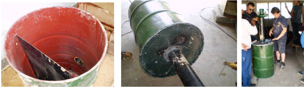
Figure 8 Ash trap and Gas Cooler assembling
