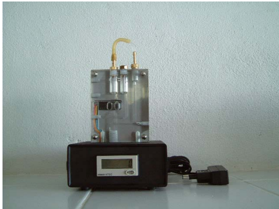
Figure 15: Gas flow meter (left: 1 st design, right: 2 nd design)
