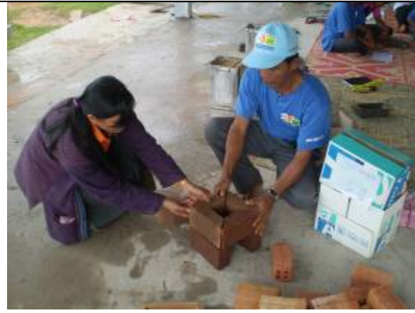
Level 2 trainer showing villager (level 3) how to assembly the rocket stove
