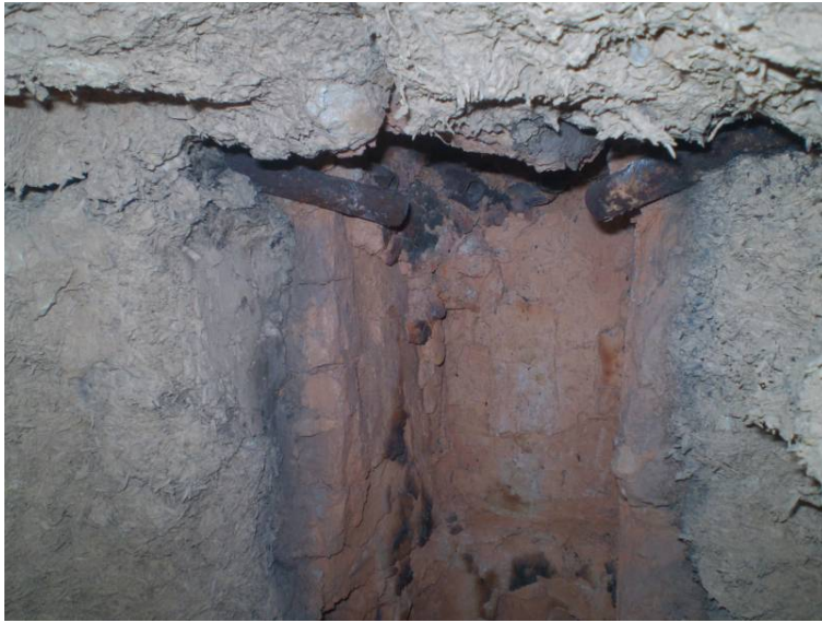
Figure 7 Air tube, disappeared (melted) reactor tube and burnt mud surround
