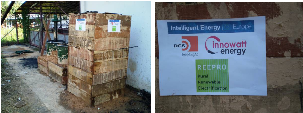
Figure 11 Constructed gasifier is running to heat up and be dried
