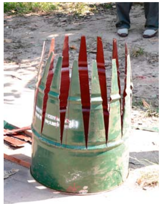
Funnel-shaped fuel silo from a 200-litre oil barrel
